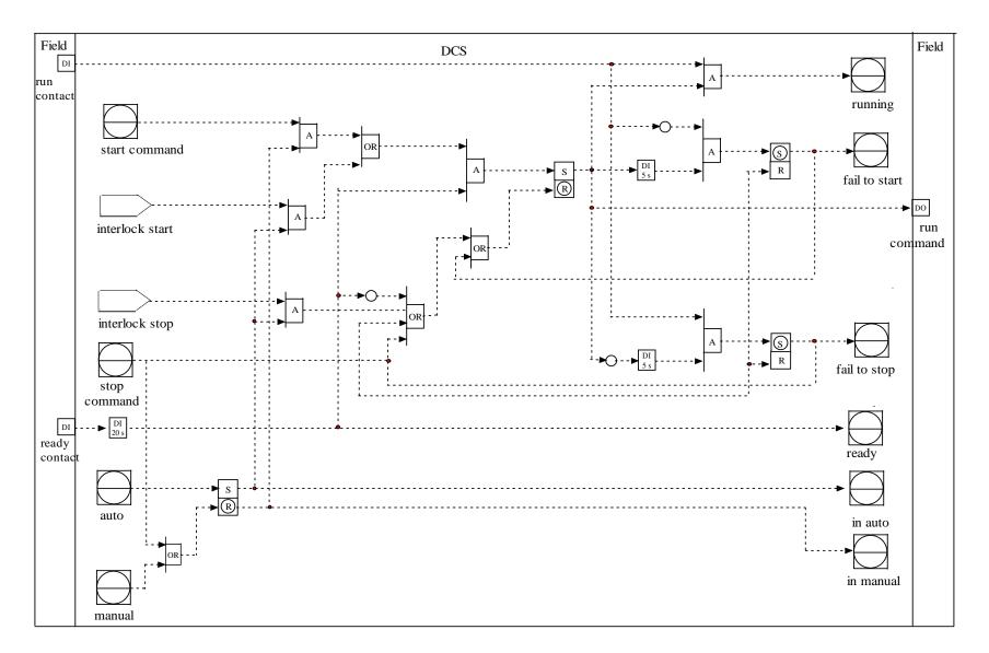
Figure 4.1.1 Agitator control logic
