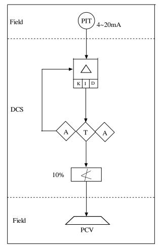
Figure 4.2.1 Back Pressure Loop Control
