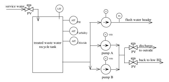
Figure 2.7.1 Treated Waste Water Recycle System
