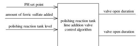
Figure 2.5.2 Polishing reaction tank lime addition valve control algorithm
