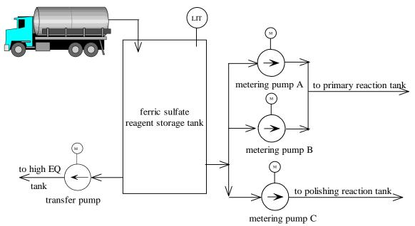
Figure 2.8.1 Ferric Sulfate Reagent Preparation System Ferric sulfate preparation system is an auxiliary system compared to the previous
