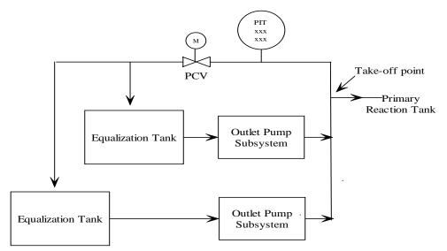
Figure 2.1.5 Equalization Tank Recycle Line Back Pressure Control The selected outlet pump is centrifugal pump. Its working discharge head is ??? psi.
