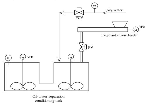
Figure 2.11.3 Coagulant Solution Preparation and Addition System Coagulant addition rate is in proportion to incoming oily water. Coagulant addition rate
