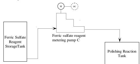
Figure 2.2.3 Polishing Reaction Tank ferric sulfate solution addition The ferric sulfate solution addition is ratio control. The amount of addition rate isproportional to the total waste water flow rate from equalization to primary reaction tank A.Other factors that affect ferric sulfate addition rate are concentration of vanadium in wastewater and selected iron to vanadium ratio. The relation between them can be expressed by thefollowing equation.
