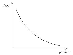
Figure 2.4.2 Filter Press Inlet Pressure-Flow Rate Relation
