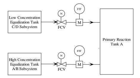
Figure 2.1.6 Equalization Tank to Primary Reaction Tank Feed Flow Rate Control The total design flow rate is 800USGPM to primary reaction tank. The operator shall
