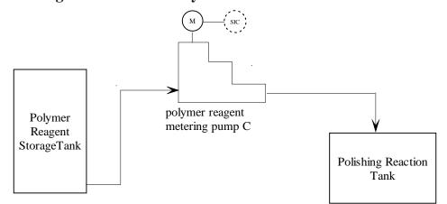
Figure 2.2.5 Polishing reaction tank polymer solution addition Addition of polymer to polishing reaction tank is used to flocculate fine suspended
