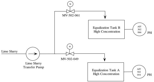
Figure 2.1.3 Equalization Tank Lime Slurry Addition
