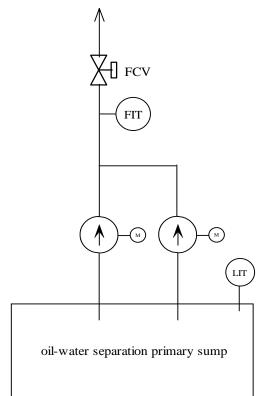
Figure 2.11.4 OWS Cartridge Filter Feed System In the OWS cartridge filter feed system, two redundant centrifugal pumps are designed
