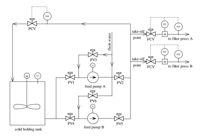
Figure 2.4.1 Filter Press Feed System
