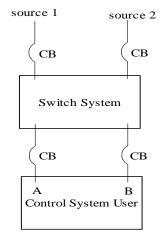
Figure 3.1.1 WWTP Power System for Control Use Figure 3.1.1 shows Power system supply for control use. Control system power supply
