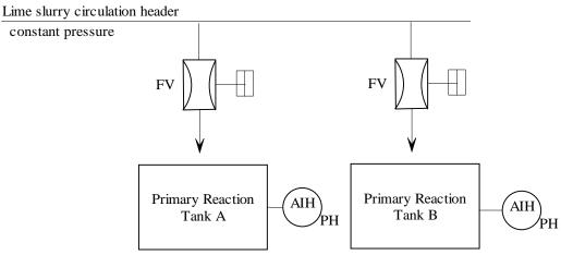
Figure 2.2.1 Primary Reaction Tank A and B lime solution addition Lime solution preparation system provides a constant pressure in the circulation header
