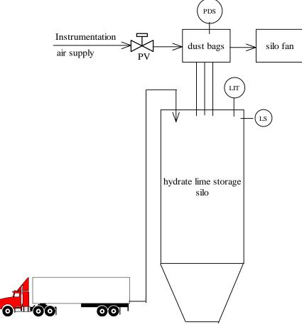
Figure 2.10.1 Lime Storage Silo System
