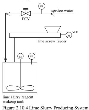
Lime slurry producing system consists of service water flow transmitter, service water flow control valve, lime screw feeder, lime slurry reagent makeup tank, agitator, and makeup
